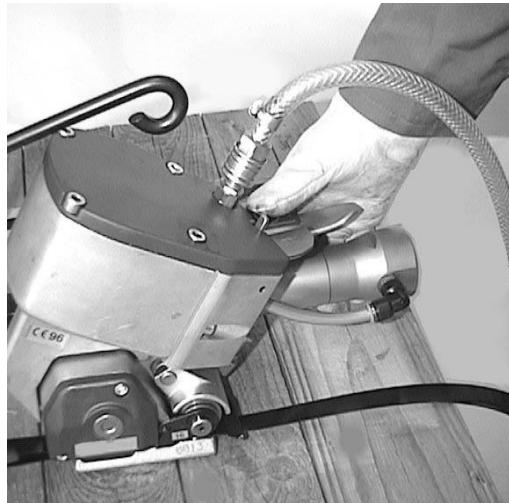
5. If the strap tension required has been achieved then the „joint“ key button **(b)** is pressed until the lock has been formed and the strap is audibly cut off behind the joint.
