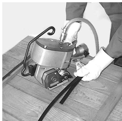
3. Hold both of the precisely overlapping straps firmly using your left hand. Using your right hand take hold of the lifting lever (c) and compressed air motor (f) and press together. Push both straps laterally along the housing wall into the tool as far as possible. A bit of the lower strap has to project out of the front of the tool. Release the lever (c) and motor (f).
