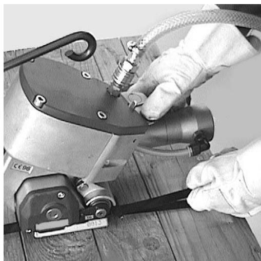
6. Take hold of strap end that is cut off with your left hand, press the air lever **(c)** and the compressed air motor **(f)** together using your right hand und swing the tool to the right out of the strapping.
