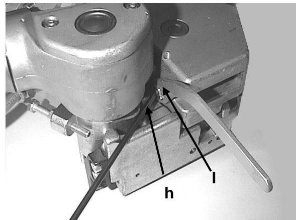
Fasten lock nut (**I**) using spanner after adjustment has been completed.
